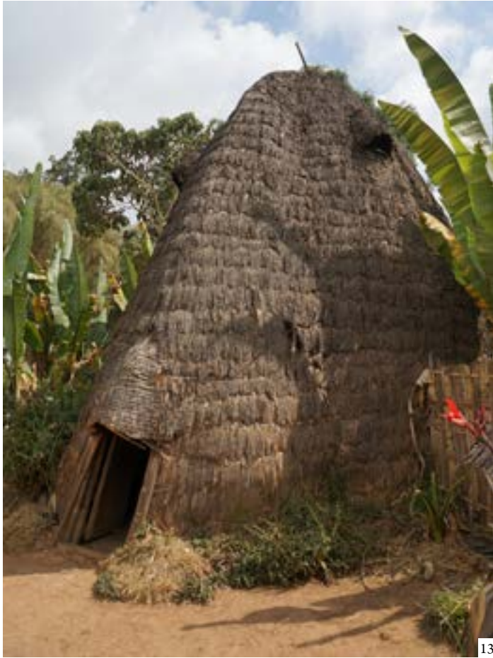
Figure 13: Dorze house made of bamboo around Arba Minch area
