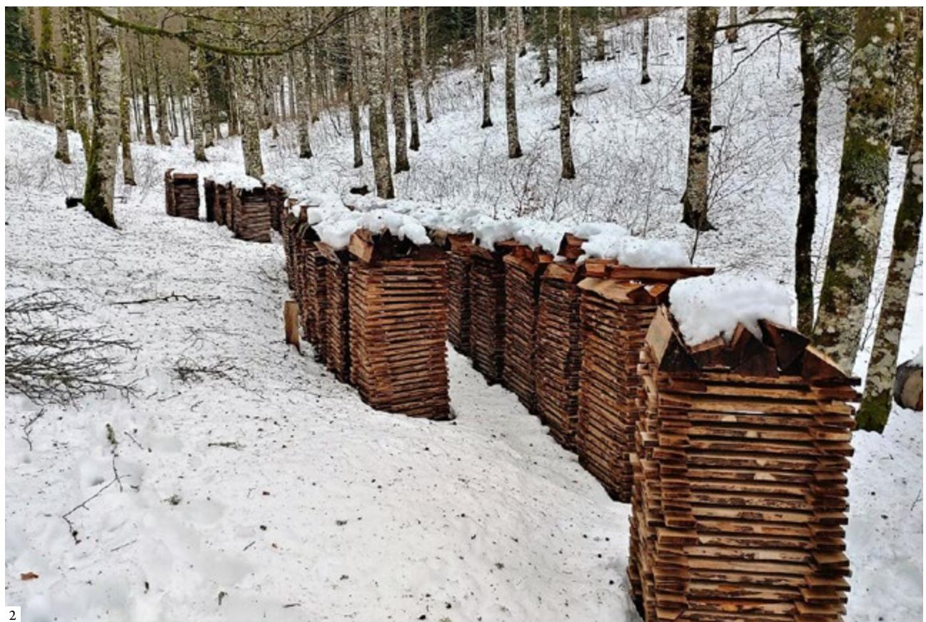
Obtaining shingles involves dividing the trunk into *trozas* or *trallos* – logs sawn at either end, 65 cm long. No more *trozas* than those that can be worked and finished in a day should be made, as if left unworked, they lose the freshness they have when recently cut. The *trozas* are taken to the site where they are to be cut, where the shingles will later be piled up for drying.
